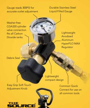
The Source HyperFLO MAX is specifically engineered for demanding applications. The newest patented regulator technology with high flow porting assures you non-freezing service with Carbon Dioxide at any delivery pressure.
